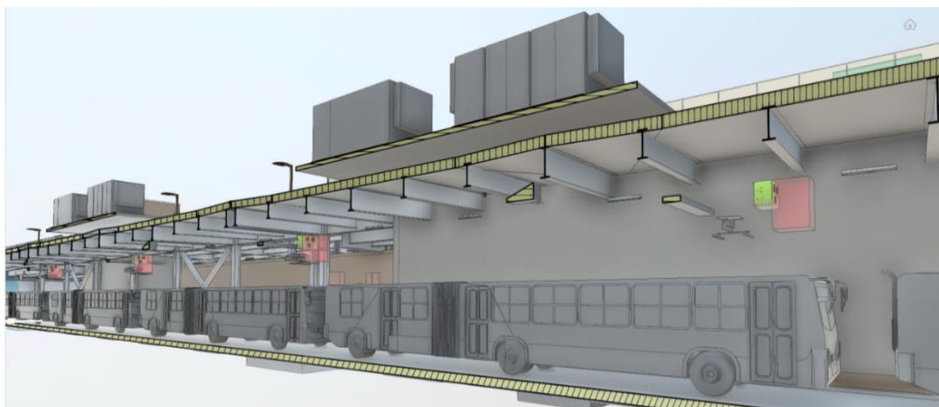
Figure 14: A rendering of BEBs with pantograph chargers overhead in the interior of the reconstructed Eastern Bus Division.
