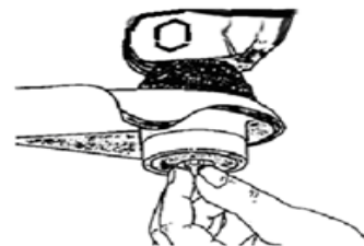
PHYSICAL INSPECTION OF "MOVEMENT" STYLE WEAR INDICATING BALL JOINT
