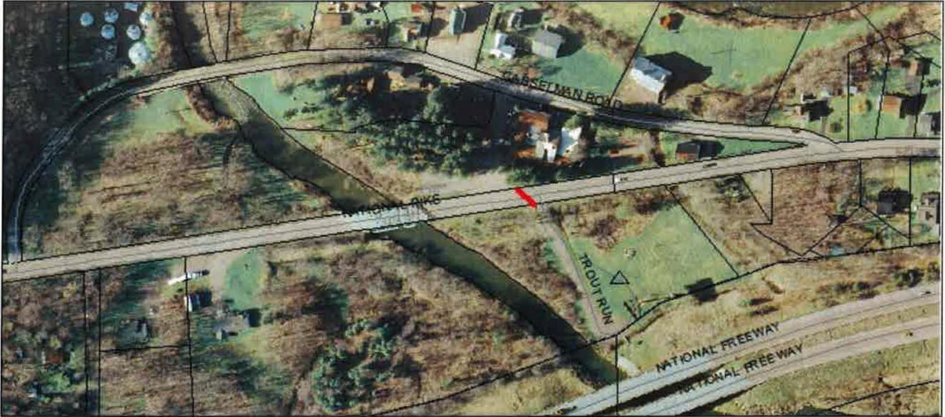
**DESCRIPTION:** The County requests a pedestrian crosswalk be installed at the location shown in red in the map above. Coordination between this project and the #2 sidewalk/streetscape project, a sidewalk from the access road for the Casselman River Bridge State Park to River Road, would be appropriate, and facilitate the sharing of resources as well demonstrate optimal project management.
